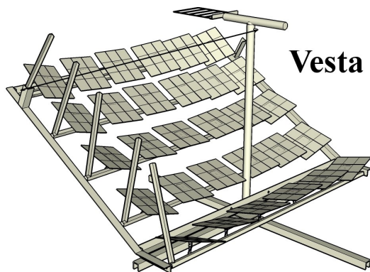
Solar Concentrator - vertical reflection - Stove Top - 400 C° - 1800 W
